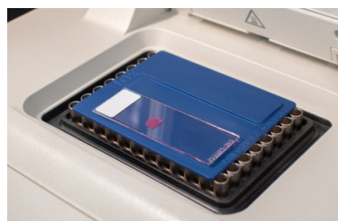
Incubation on a Thermal Cycler
