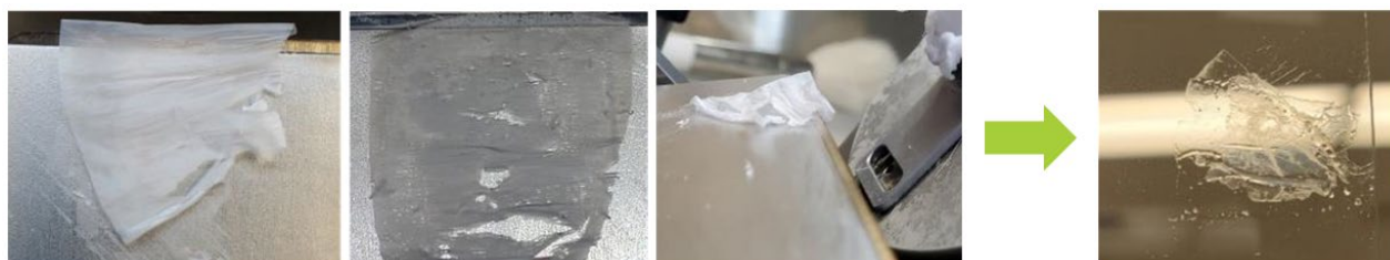
Figure 8. Consequences of mounting imperfect sections
