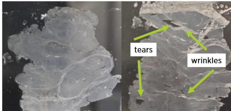
Figure 9 - Good (left) and bad (right) sections mounted on a slide
